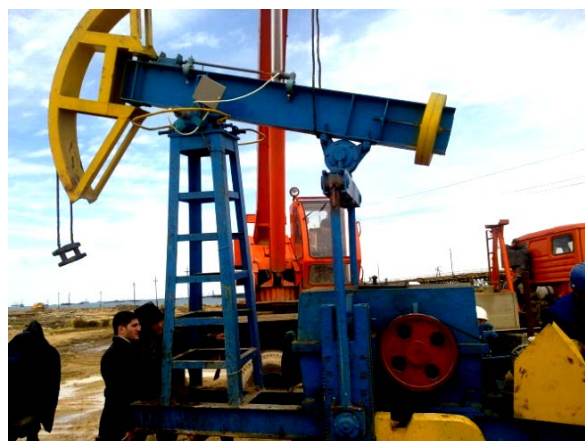
Fig.3. Mechanical drive rod pumps for oil well depth of 720 meters in relation to the SKD 3-1,5-710 with the new double-flow constructive three-stage cylindrical gear reducer U_{\Sigma}=64 .
