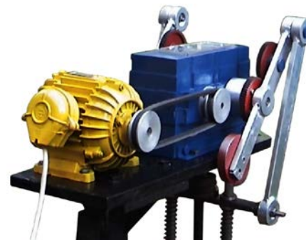
Fig. 2. Mechanical drive rod pumps for water wells depth of 40 meters with a new constructive solution double-flow three-stage cylindrical gear reducer with a gear ratio U_{\Sigma}=64 .
