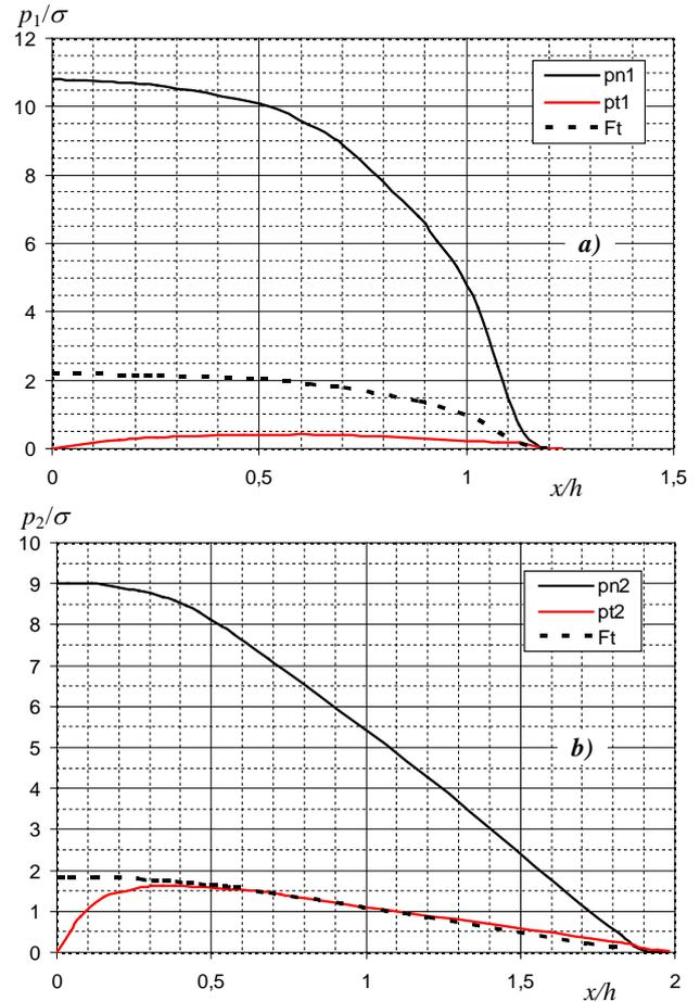
Fig. 4. Contact pressure distributions for  $R/h = 50$ : a) at the indenter-layer interface  $a/h \approx 1.24$ ,  $p_{n1,max}/\sigma \approx 10.8$ ; b) at the layer-substrate interface  $b/h \approx 1.99$ ,  $p_{n2,max}/\sigma \approx 9$
