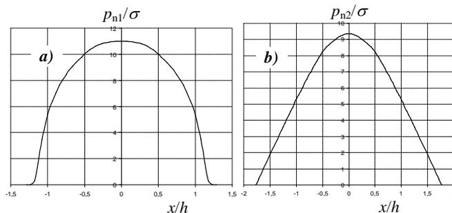
Fig. 3. Contact pressure distributions for the frictionless case and geometry  $R/h = 50$ : a) at the indenter-layer interface  $a/h \approx 1.29$  and  $p_{n1,max}/\sigma \approx 11$ ; b) at the layer-substrate interface  $b/h \approx 1.78$  and  $p_{n2,max}/\sigma \approx 9.35$
