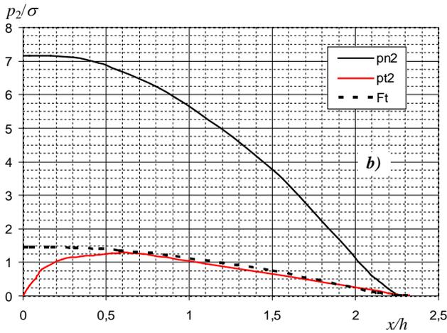
Fig. 5. (continued) Contact pressure distributions for  $R/h = 100$ ; b) at the layer-substrate interface  $b/h \approx 2.32$ ,  $p_{n2,max}/\sigma \approx 7.16$
