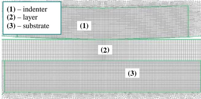
Fig. 2. Mesh detail around the initial point of contact
