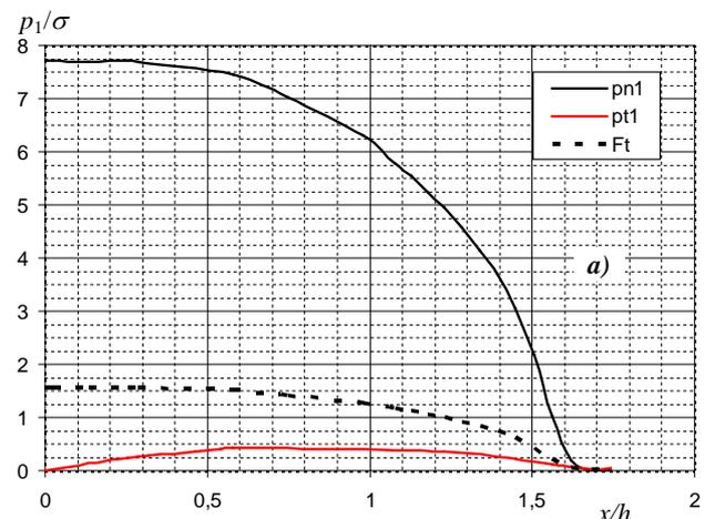
Fig. 5. Contact pressure distributions for  $R/h = 100$ : a) at the indenter-layer interface  $a/h \approx 1.74$ ,  $p_{n1,max}/\sigma \approx 7.71$
