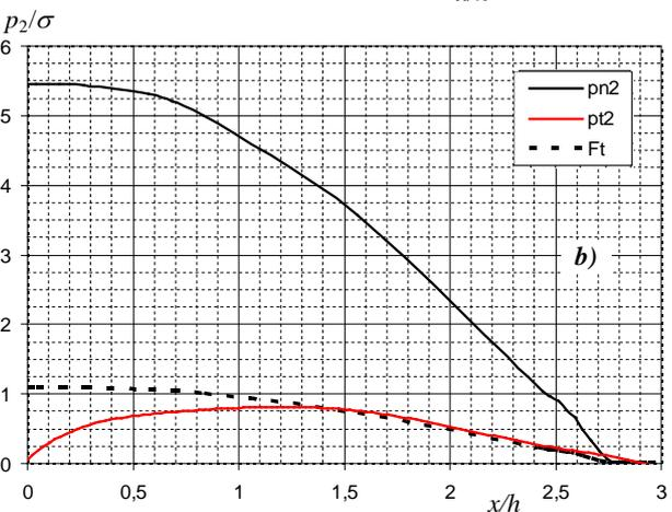
Fig. 6. Contact pressure distributions for  $R/h = 200$ ; a) at the indenter-layer interface  $a/h \approx 2.41$ ,  $p_{n1,max}/\sigma \approx 5.4$ ; b) at the layer-substrate interface  $b/h \approx 2.97$ ,  $p_{n2,max}/\sigma \approx 5.45$
