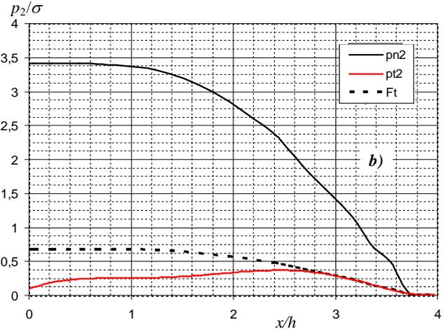
Fig. 7. Contact pressure distributions for  $R/h = 500$ ; a) at the indenter-layer interface  $a/h \approx 3.97$ ,  $p_{n1,max}/\sigma \approx 3.46$ ; b) at the layer-substrate interface  $b/h \approx 3.98$ ,  $p_{n2,max}/\sigma \approx 3.42$
