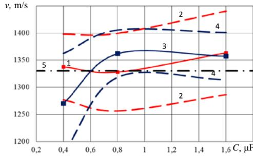
**Fig. 4** Velocity of pressure wave front during HVED with the use of kerosene as continuous medium
