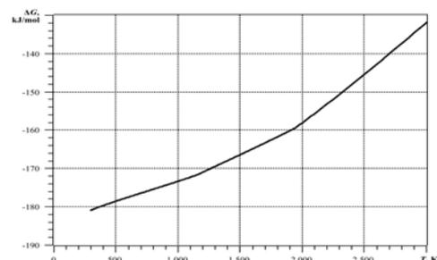
Fig. 1 Dependence of Gibbs energy change of  $Ti + C \rightarrow TiC$  reaction on temperature
