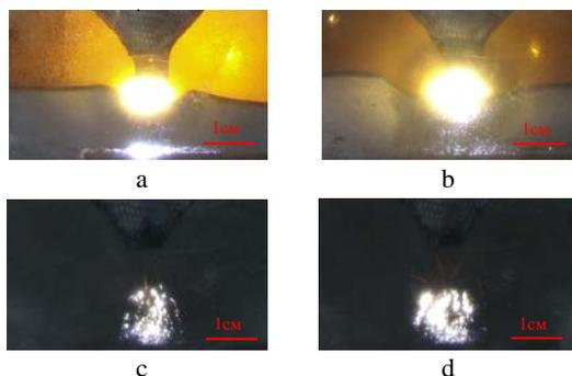
**Fig. 2** Integral photos of discharge in “Ti powder – kerosene” disperse system with single discharge energy  $W_d = 90\ \text{J}$  and initial dispersity  $d_m = 100\ \mu\text{m}$  after 5<sup>th</sup> (a), 10<sup>th</sup> (b), 50<sup>th</sup> (c) u 100<sup>th</sup> (d) pulses
