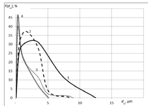
**Fig. 8** Distribution of percent content  $F(d_m)$  of Ti powder particles by values of mean diameter  $d_m$  after HVED treatment with specific energy  $W_{sp}$  10 (1), 20 (2), 30 (3) and 40 MJ/kg (4)
