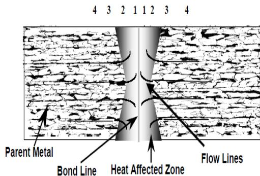
Fig.4 Schematic illustration of constitutive parts of weld area
