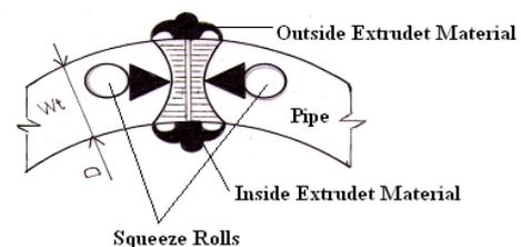
Fig.2 Effect of plastic deformation on the HFERW
