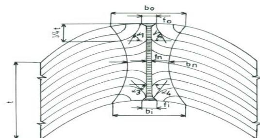
Fig.3 Flow lines (fibres) and flow angles around bond line during plastic deformation
