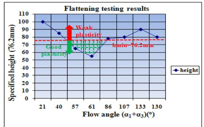
Fig.10 Plasticity of the welded joint
