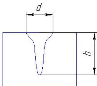
Fig. 1 – Schematic representation of the joint weld depth and width
