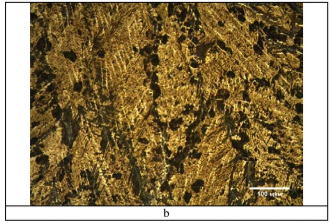
Fig. 5 – Microstructure of 40X joint welds obtained by EBW without preheating (a) and (b)
