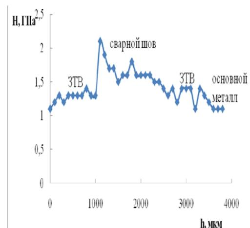
Fig. 4 – Microhardness distribution in 40X joint weld produced by EBW
