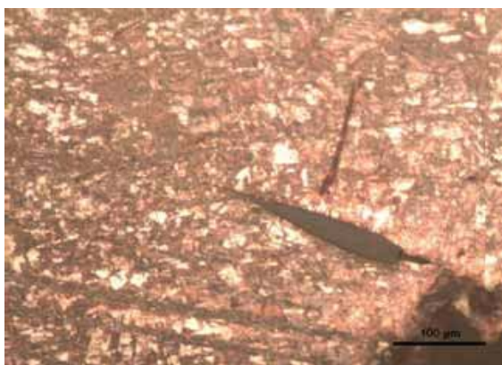
Fig.10 Non-metallic inclusion in the area of welding
