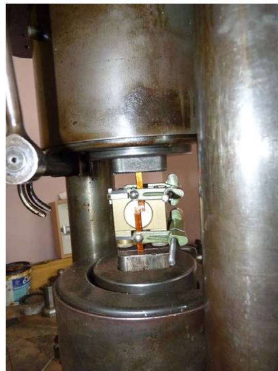
Fig.2 Recording the extension during the sample demolition for creating a stress-strain diagram.
