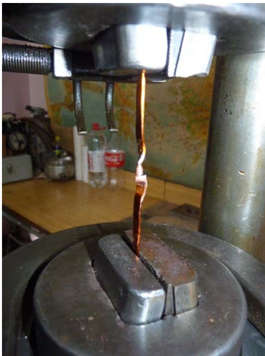
Fig.1 Destruction process of the samples on the test machine to determine the strength of the welded joint.
