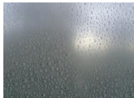
Fig.5. A microphotograph of a transparent conductive film formed from the OS and Silvernano-1 solution.
