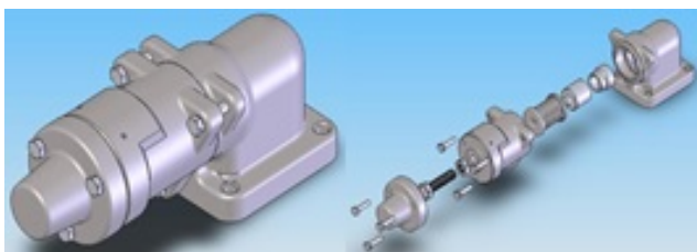
Fig. 2 Safety – overflow valve
