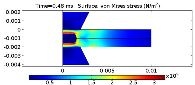
Fig. 2 Distribution of von mises stress at the end of welding time
