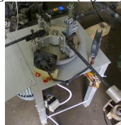
Figure 1 Stand for accelerated wear test under dry friction
