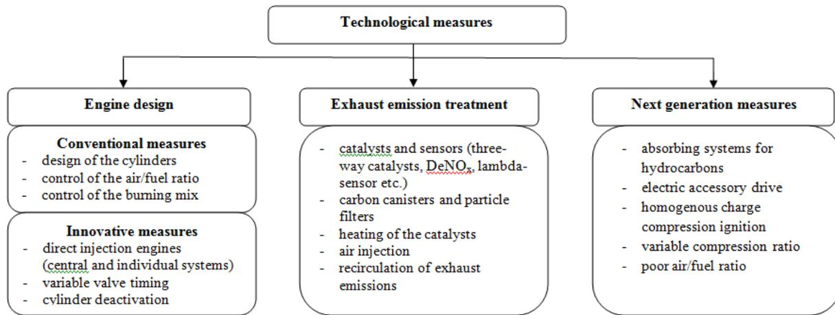
Fig. 2: Categorization of technological measures at vehicles
