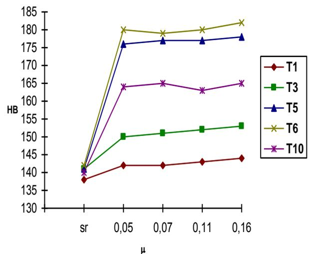
Fig. 6. Brinell hardness HB measured in different points T as a function of lubricant's coefficient of friction  $\mu$  (sr. = unformed alloy)
