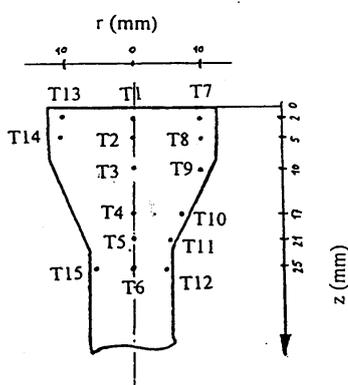
Fig. 5. Measuring points for Brinell hardness
