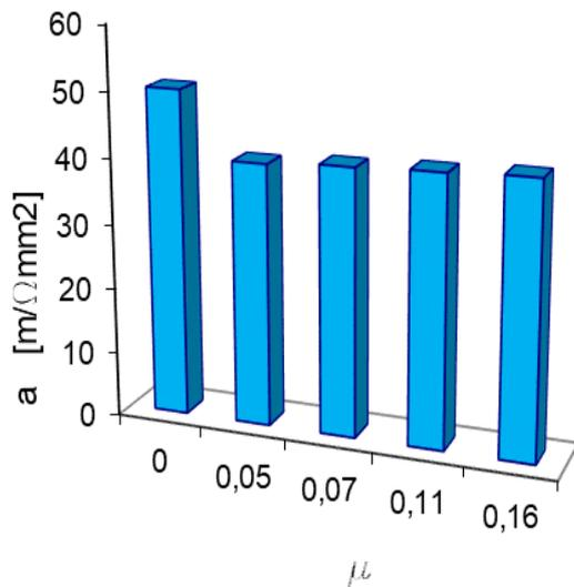
**Fig. 7.** Effect of coefficients of friction on electrical conductivity  $a$  of the extruded specimens (No. 0 on x-axis represents the value of unformed alloy)
