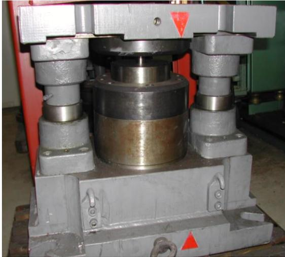
Fig. 1. Experimental tool for cold forward extrusion
