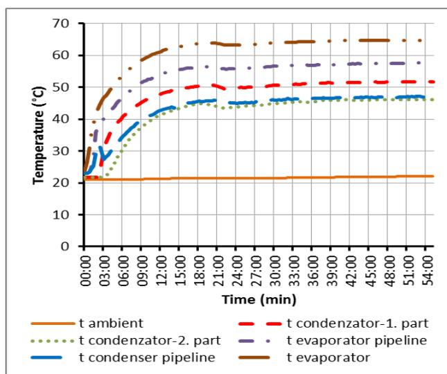
Fig. 9 Results of the loop thermosiphon temperature measurement
