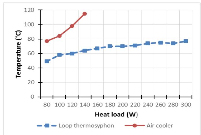
Fig. 10 Temperature development depending on the heat load
