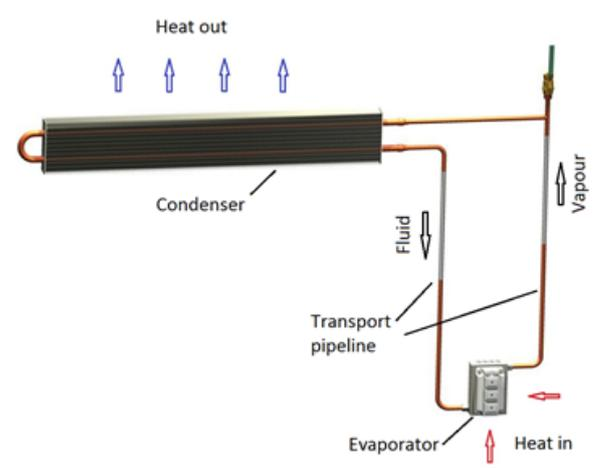
Fig. 1. Loop thermosiphon model
