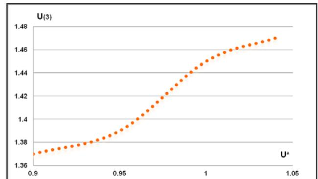
Fig. 3 Dependence of the percentage of the third harmonic U(3) from the relative value of the voltage U\*.
