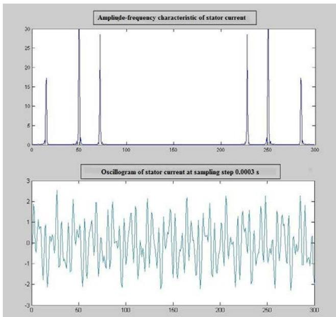
Fig. 4. Amplitude-frequency characteristic and oscillogram of stator current
