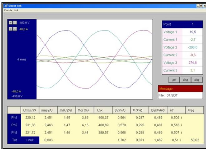
Fig. 1 Voltages and currents measured of the three-phase induction motor type ATM 100L4
