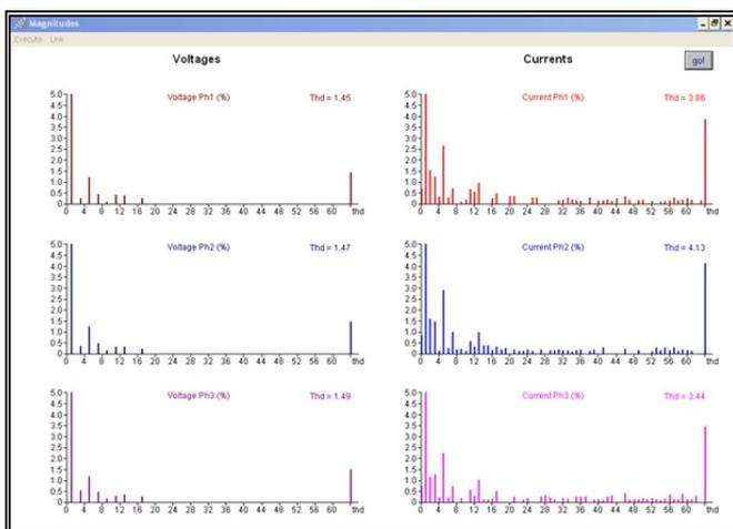
Fig. 2 Harmonics composition of the voltages and currents measured
