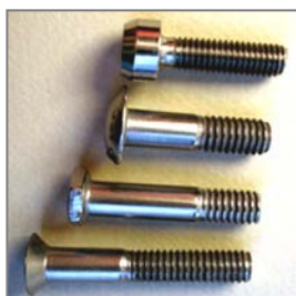
Fig. 9. Bolts produced from high-strength and corrosion-resistant nitrogen containing steel 05Kh16N5AB by cold upsetting technology
