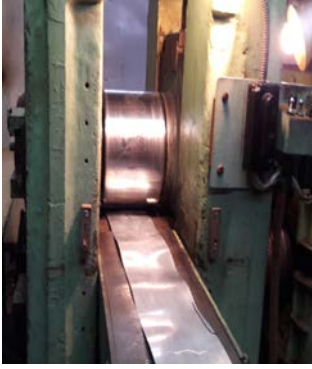
Fig. 7. Rolling unit Mill DUO-280 (Rubin company, Kharkov)
