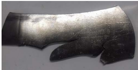
Fig 3. Common view of the billet after compression more than 10 % during hot rolling at 1100 °C
