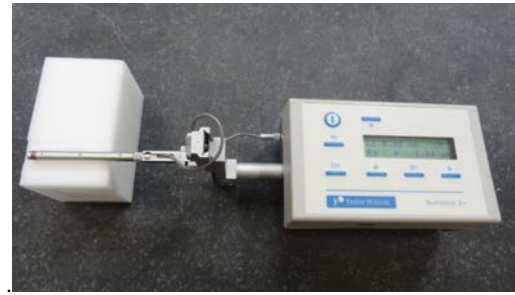
Fig. 7 Surface roughness measurement using roughness meter Surtronic3+
