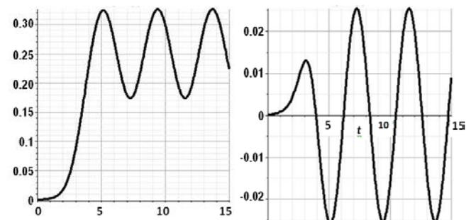
Fig.11. Lifting cable - Velocity  $v(z)$  and angular velocity  $w(z)$
