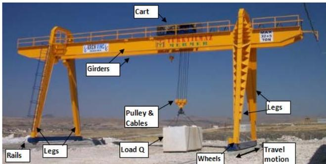
Fig.1. Gantry crane with parts [1]
