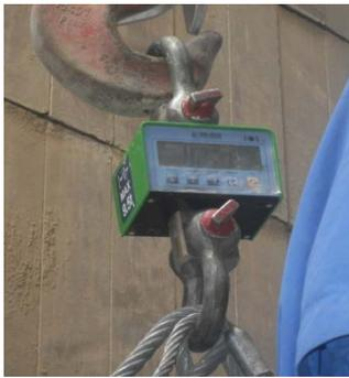
Fig.5. Measurements with Dynamometer during motion of crane
