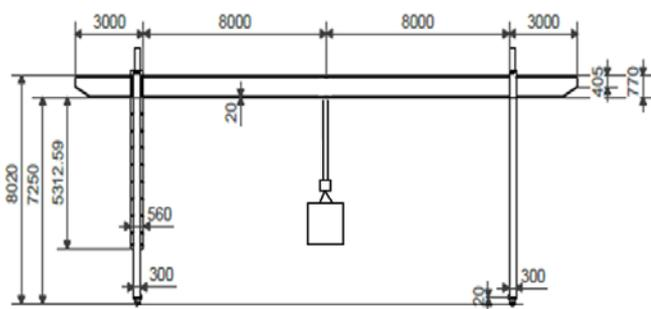
Fig.2. Gantry crane main dimensions [1]
