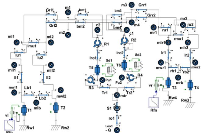
Fig.3. Block Diagram of gantry crane with travel motion
