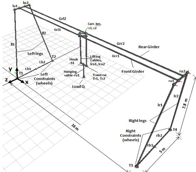
Fig.4. Discrete-continuous model of gantry-crane
