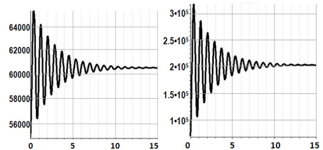
Fig.16. Torque  $T(x)$  and  $T(z)$  in Crane's Front Girder
