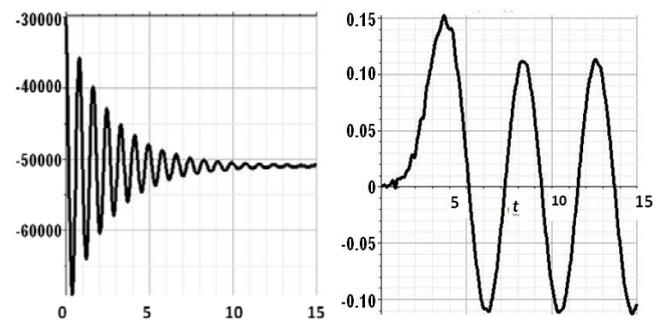
Fig.10. Lifting cables – Force  $F(y)$  and Acceleration  $a(z)$
