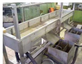
Fig. 24. NO-180 pilot ultrasonic unit for ground decontamination
