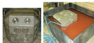
Fig. 23. Ultrasonic decontamination of fluid radioactive waste storages
