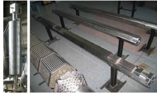
Fig. 3. Ultrasonic cleaning equipment for NPP fuel assemblies with VVER
