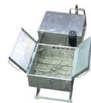
Fig. 22. MO-12 ultrasonic decontamination unit
