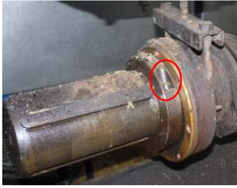
Figure 2 Appearance of damaged reducers half-ring.
