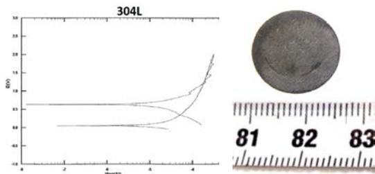
Figure 5 Cyclic polarization diagram and macro recording of sample 304L.
