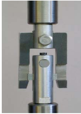
Fig. 4 Modified bending tests (notch toughness test).
