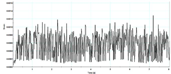
Fig.10. Strain Von Misses in main girder
