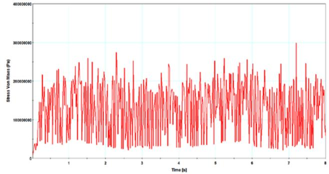
Fig.9. Stress Von Misses in main girder
