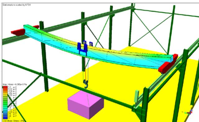
Fig.8. Deformation of main girder (Scaled by 6.274), and contour spread of Von Misses Stress
