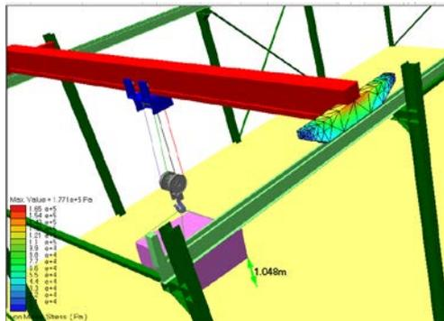
Fig.13. Contour spread of Von Mises stress in right side girder
