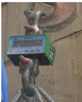
Fig.6. Measurements with Dynamometer during motion of crane
