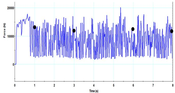
Fig. 7. Tensile force  $F_t$  in one branch of lifting cable. Black dots are experimental values from Table 1.
