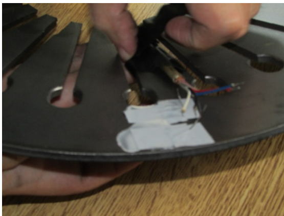
Fig.10a. Diaphragm spring with measuring tapes
