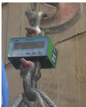
Fig.6. Measurements with Dynamometer during motion of crane
