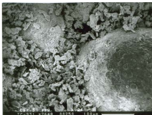
Fig. 11 Surface of the experimental sample when the thin permeable layer is applied
