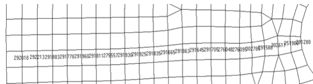
Fig. 6. Network of spring calculation. The network of the spring is divided into 21 parts and for each part is measured the stress on the underside of the spring.
