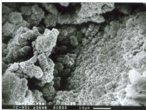
Fig. 13 The coating on the substrate particle (on the right) and on the removable agent (on the left)
