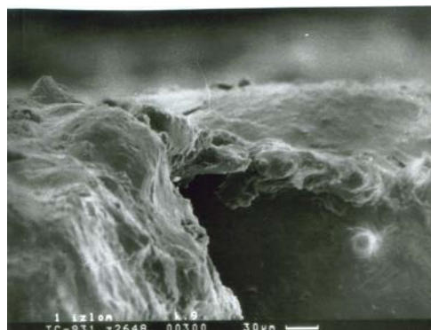
Fig. 10 Fractogram of the brittle fracture of the experimental sample in the region of the removable agent at various magnifications: a) \times 250 ; b) \times 300
