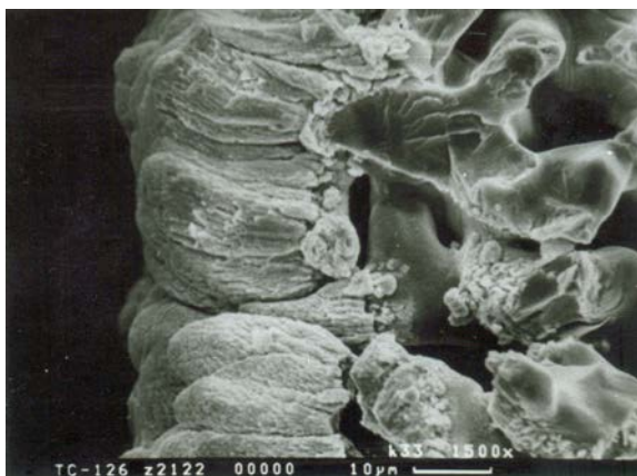
Fig.1 The structure of the PPM produced by ion-plasma sputtering method in a vacuum without a removable agent
