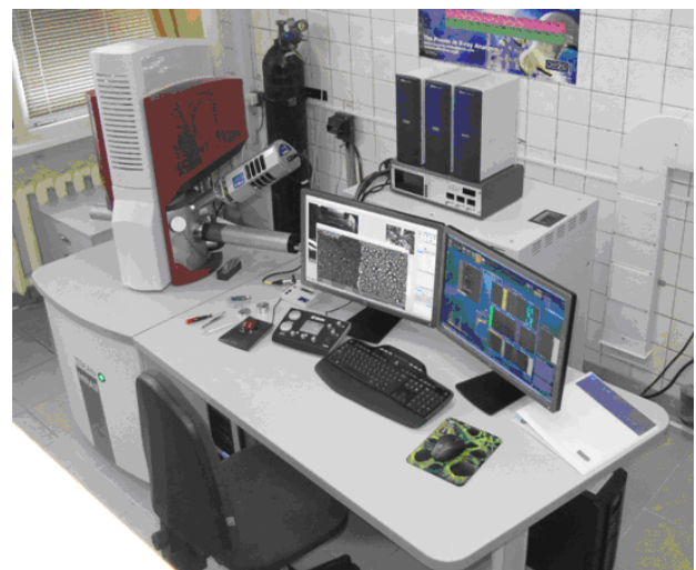
Fig. 2 A high-resolution scanning electron microscope "Mira-3" of Tescan company (Czech Republic)
