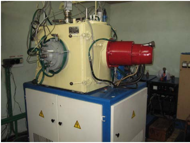
Fig.3 A vacuum machine HHB-6.6-III for the application of vacuum composite functional coatings
