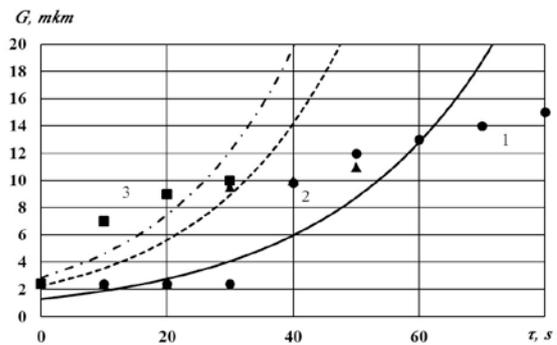
Fig. 5 Experimental values of grain size in consolidated Fe powder specimens after SPS with different heating rate and curves of their approximation
