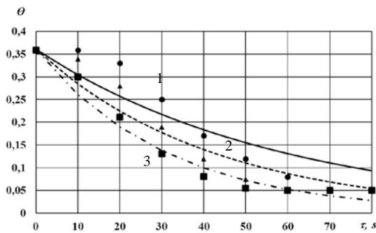
Fig. 3 Experimental curves of changes of porosity of consolidated Fe powder specimens after SPS with different heating rate
