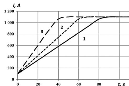
Fig. 1 Experimental curves of changes of current amplitude during SPS with different heating rate
