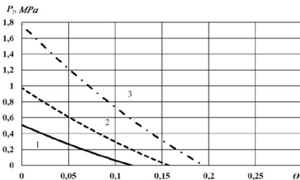
**Fig. 10** Theoretical curves of changes of capillary pressure depending on porosity of consolidated Fe powder specimens after SPS with different heating rate
