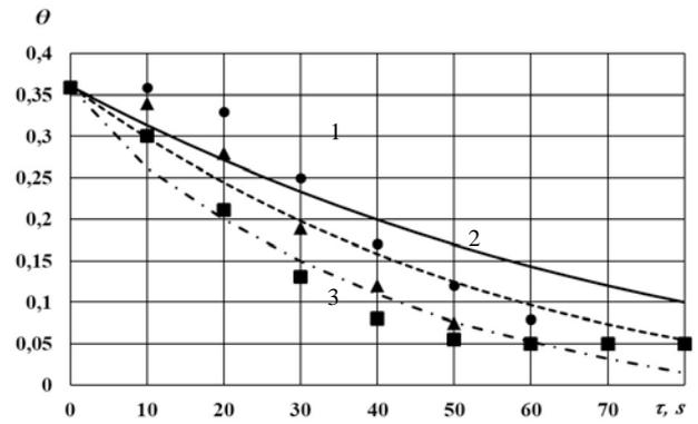
**Fig. 8** Experimental values and theoretical curves of changes of porosity of consolidated Fe powder specimens after SPS with different heating rate
