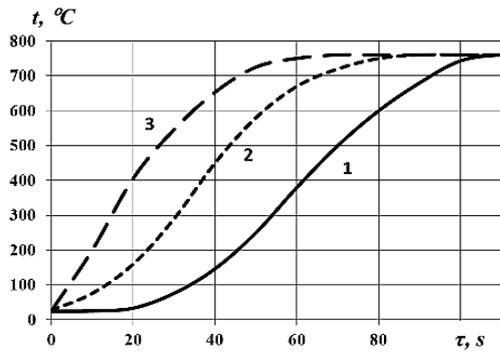
Fig. 2 Experimental curves of changes of temperature during SPS with different heating rate
