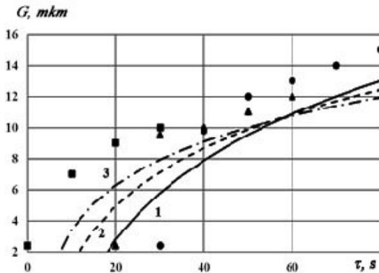
**Fig. 7** Experimental values and theoretical curves of grain size in consolidated Fe powder specimens after SPS with different heating rate
