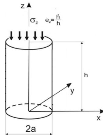
**Fig. 9** Model of densification of cylindrical specimen in hard matrix under external axial pressure
