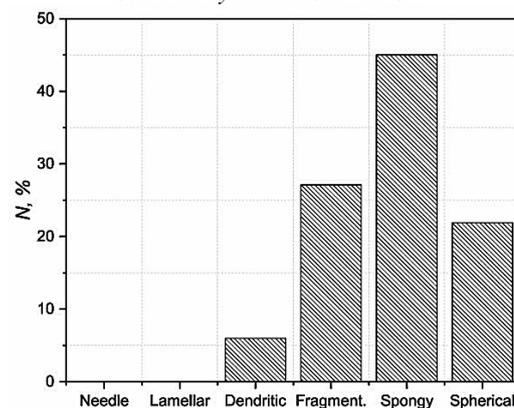
Fig. 2. Form distribution of powder particles of the Ti-Al-C system obtained by mechanoactivation
