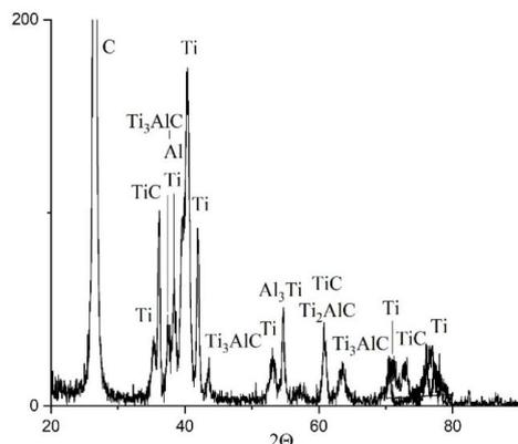
**Fig. 8.** Phase composition of the SPS-consolidated HVED-activated powder,  $\text{CuK}\alpha$ -radiation
