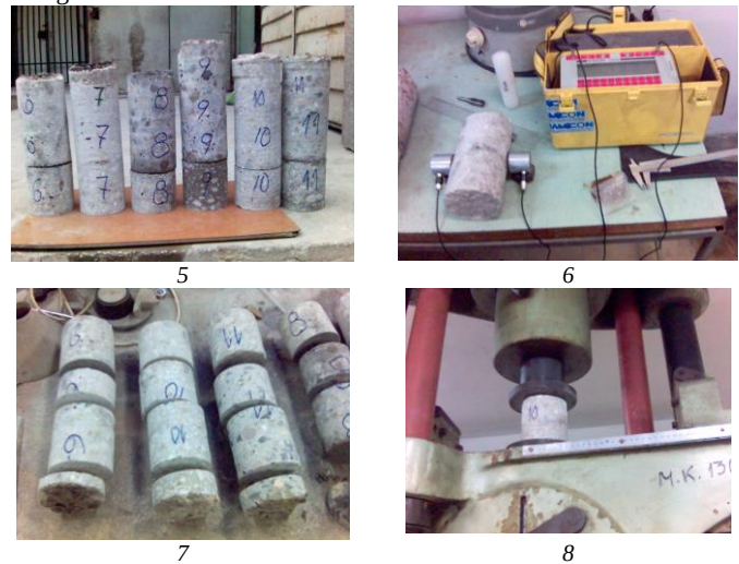
Photos 5, 6, 7 and 8 Core cutting, preparing and testing
