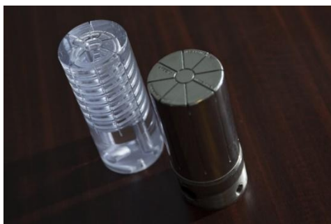
Fig. 3.2 A Bastech mold core insert with conformal cooling channels prototyped using 3D Systems' Stereolithography (SLA) technology and printed in maraging steel on the ProX® DMP 200. (Source: 3dsystems.com)
