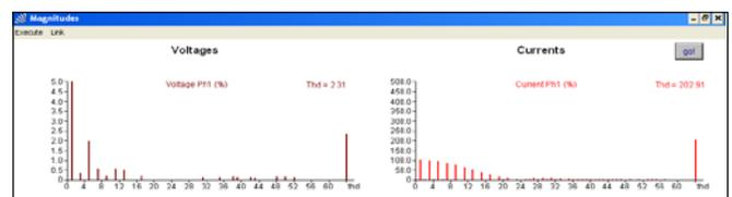
Fig. 5 Observed harmonics for centrifugal fan at frequency of 30 Hz
