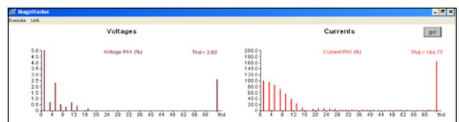
Fig. 4 Observed harmonics for centrifugal fan at frequency of 50 Hz
