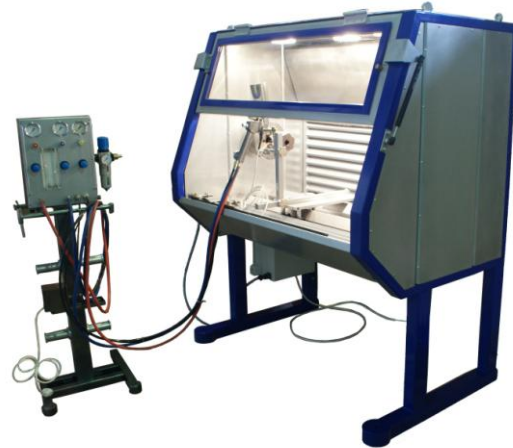
Fig. 4. Chamber of semi-automatic spraying TENA-KPAN-1300 with the equipment of gas-flame spraying TENA-Ppm
