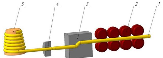
1 – wire; 2 – pushing device; 3 - equal channel step matrix; 4 – calibrating drawing tool; 5 - winding drum
