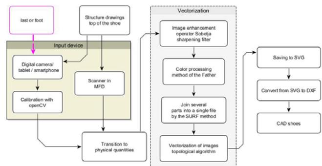
Fig. 4 Structural-logic diagram of the vectorization block.
