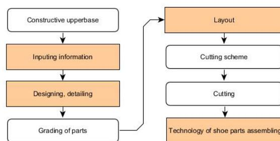
Fig. 1 Structural-logical scheme of designing shoes.
