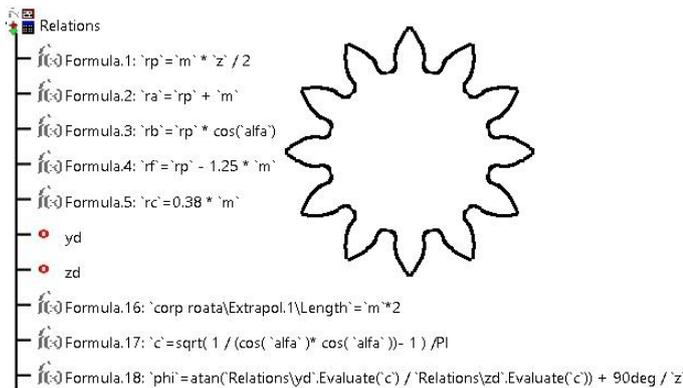
Fig. 1. Parametric creation of the gears profile
