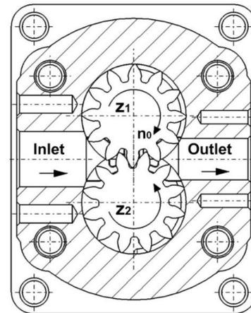
Fig. 2. Section through the gear pump
