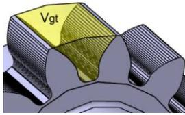
Fig. 4. The cup volume between two successive teeth
