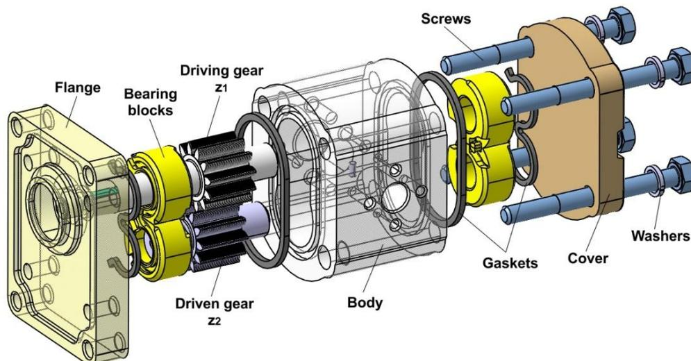
Fig. 3. The 3D model of the gear pump
