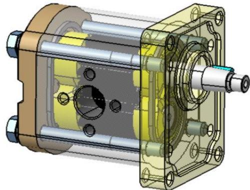
Fig. 8. Pump assembly for  $V_g=26 \text{ cm}^3/\text{rev}$
