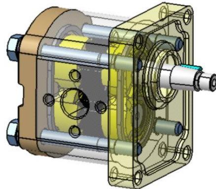
Fig. 7. Pump assembly for  $V_g=11 \text{ cm}^3/\text{rev}$
