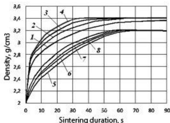
**Figure 1.** Compression kinetics of a powder composition, at sintering under high pressure conditions ( $p = 8$  GPa):  $\text{BN}_w +$  static synthesis diamonds at  $T = 1500^\circ\text{C}$  (1);  $T = 1600^\circ\text{C}$  (2);  $T = 1700^\circ\text{C}$  (3);  $T = 1800^\circ\text{C}$  (4) and  $\text{BN}_w +$  dynamic synthesis diamonds at  $T = 1500^\circ\text{C}$  (5);  $T = 1600^\circ\text{C}$  (6);  $T = 1700^\circ\text{C}$  (7);  $T = 1800^\circ\text{C}$  (8).
