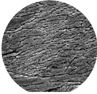
Fig. 2. The microstructure of the deformation zone after the third pass, \times 3000
