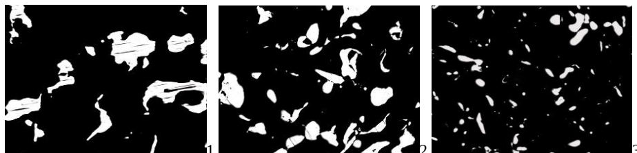
Fig. 5. Microfractograph of the powders of gray cast iron 3.5% C of different fractions, \mu m ( \times 25 ). 1) +800-1000; 2) +500-800; 3) +200-500
