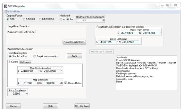
Figure 3. Topographic data generation from the SRTM Database.
