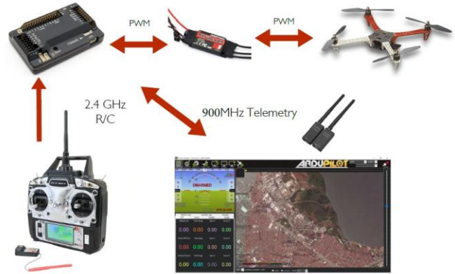
Figure 5: Communication process between quadrotor different parts.
