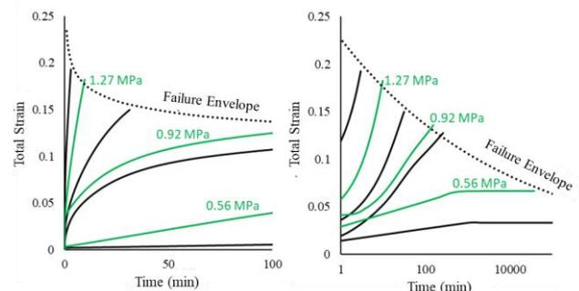
**Fig. 5** FE creep modelling for intermediate stress levels
