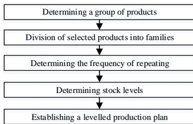
Fig. 1. Production levelling methodology, source: own
