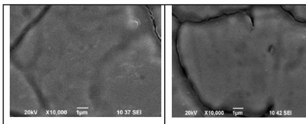
Fig. 2. Morphology of fresh coatings A3 (left) and after corrosion (right)
