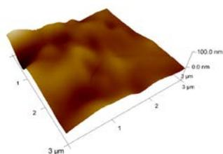
Fig. 3. AFM image (3D) of surface of fresh coating A3
