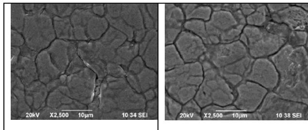
Fig. 5. Morphology of coatings A3 ( left) and A5 (right) after corrosion (right)
