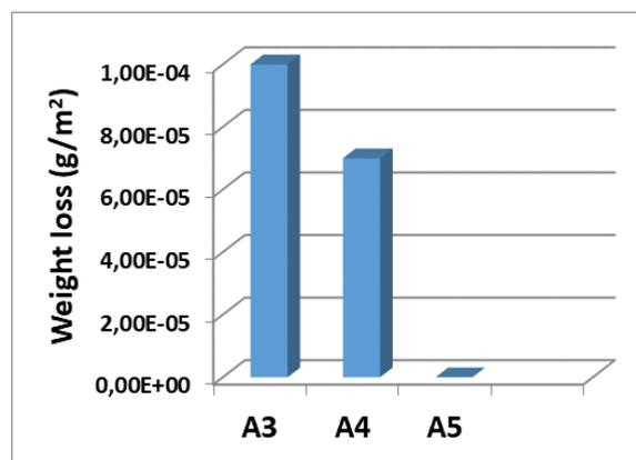
Fig. 6. Weight loss of the coatings after immersion in salt medium
