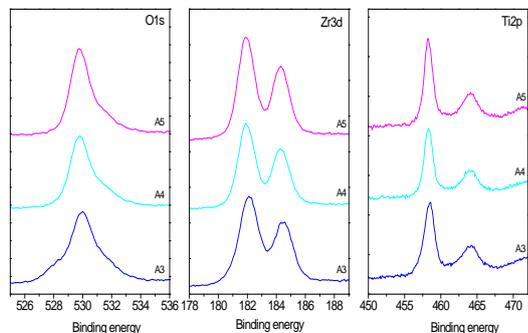
Fig. 1. O1s, Zr3d, Ti2p core level spectra of the coatings
