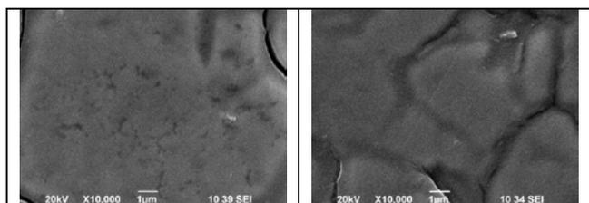
Fig. 4. Morphology of fresh coatings A5 (left) and after corrosion (right)
