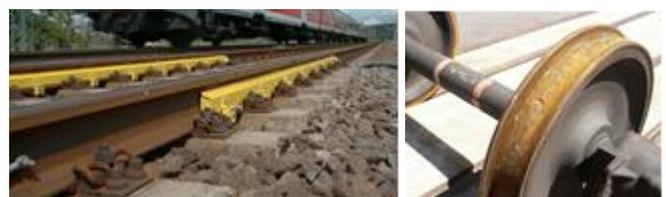
Fig. 6 Detector for entrenched wheels [12]
