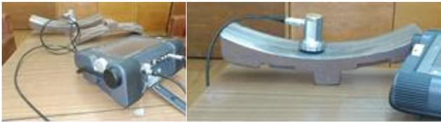
Fig. 7 Measurement with an ultrasonic flaw detector
