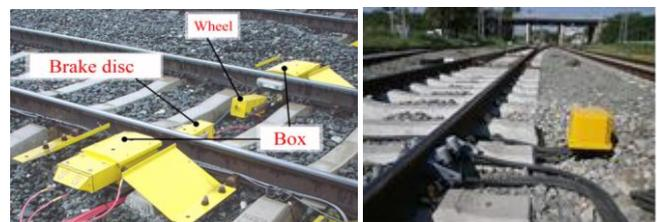
Fig. 4. Schematic diagram of the universal control point "check point" and a counter axle [12]
