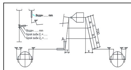
Fig. 2 Schematic diagram for the calculation of mechanical braking force for a two-axle wagon with a load of 20 t per axle with full / empty mechanical switch [1]
