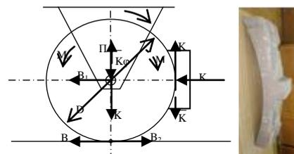
Fig.1 Occurrence of mechanical brake force [7, 8]
