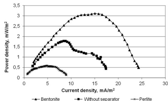
**Fig. 4** Polarization curves of SMFC-s with different substrate
