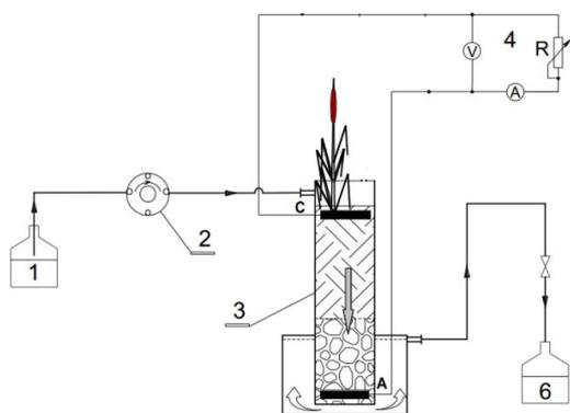
**Fig. 2** Design of Plant sediment microbial fuel cell 2
