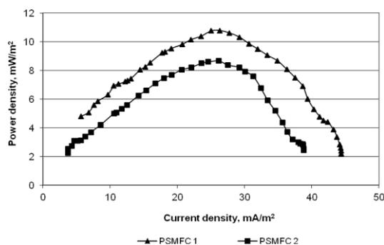
Fig. 6 Polarization curves of PSMFC-s in downstream flow mode
