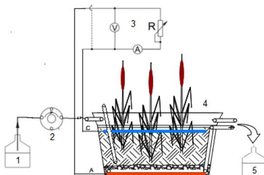
**Fig. 1** Design of Plant sediment microbial fuel cell 1
