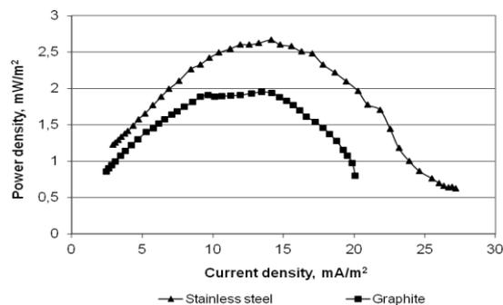
Fig. 5 Polarization curves of PSMFC-s with different electrode materials
