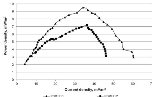
Fig. 7 Polarization curves of PSMFC-s in upstream flow mode
