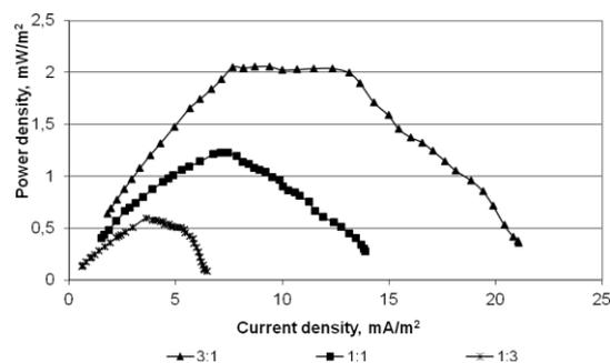
**Fig. 3** Polarization curves of SMFC-s with different ratio of sediment and peat in substrate
