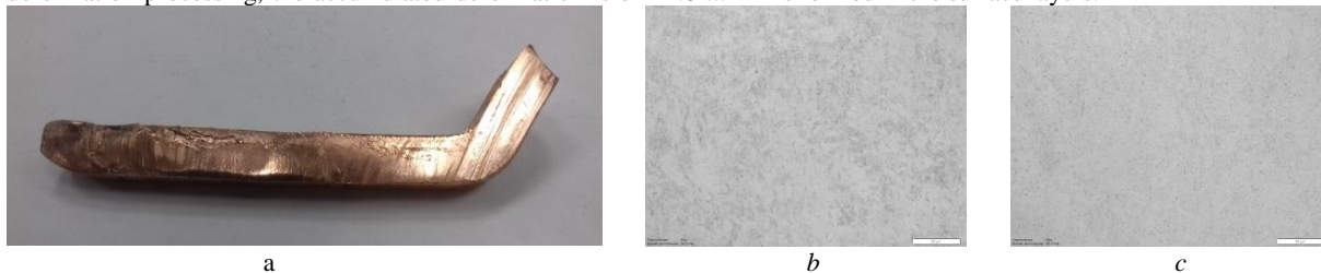
Figure 5. a - general view of the sample in the process of active bending, b - the structure of the middle zone of the cross section of the sample (OM), c - the structure of the surface area of the cross section of the workpiece (OM)
