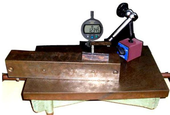
Fig.3. Experimental installation for reading the deviations in the shape
