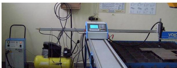
**Fig.1** Outlook of plasma cutting equipment for metals
