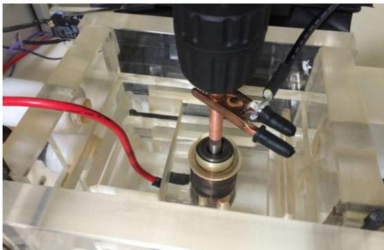
Fig. 2 Machining chamber with workpiece and tool.
