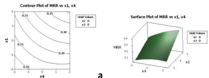
Fig. 4 Surface and Contour Plot of MRR: MRR: Voltage ( $x_1$ ) and Concentration ( $x_4$ ).
