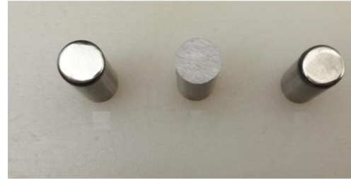
Fig. 3 Workpiece after and before machining.
