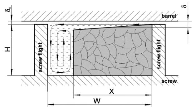
Fig. 4 The screw channel cross-section in the melting zone ( $\delta$  – average thickness of the polymer melt layer)
