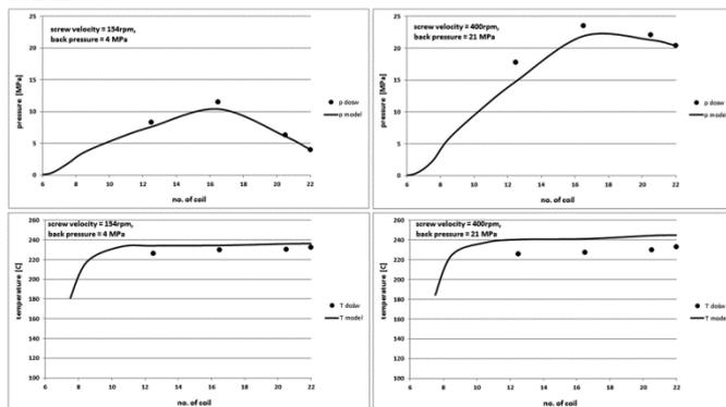
**Fig. 6** Comparison of the theoretical and experimental characteristics of the pressure (top) and temperature profiles (bottom) on the screw channel length in PP injection process for the screw rotational velocity of 154 rpm and back pressure of 4 MPa (left) and 400 rpm and 21 MPa (right)
