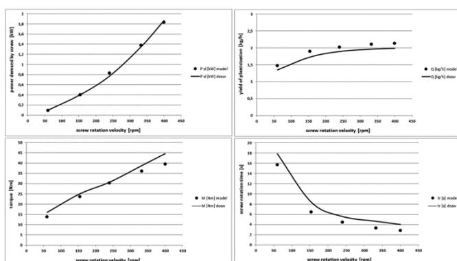
**Fig. 7** Comparison of the other theoretical and experimental characteristics (power demand, torque, yield of plasticization and screw rotation time) for the different screw rotation velocity and back pressure values in PP injection process
