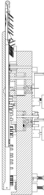
*Fig. 3* Two-dimensional section of the knitting carriage, needles and needle bed.
