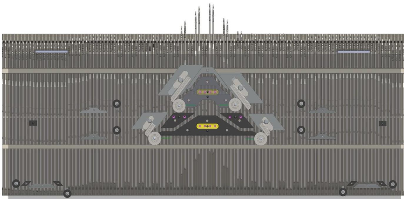
**Fig.2** Realistic three-dimensional image of the knot needle bed assembly, needle knitting mechanism in a 2x2 ribbing trajectory
