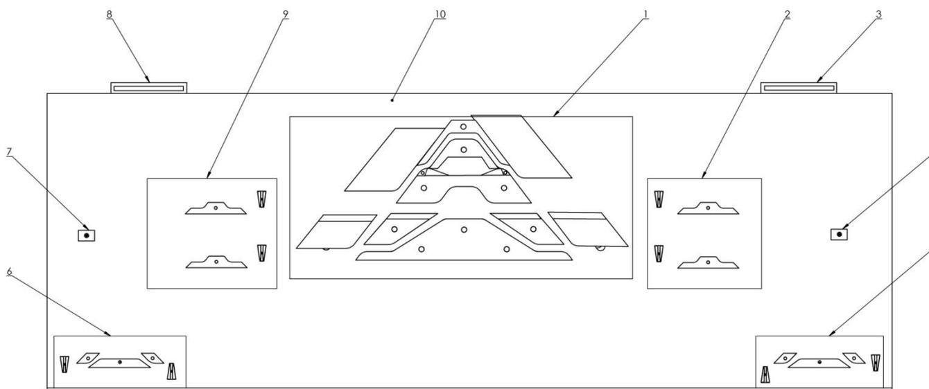
Fig.1 Knitting carriage with the complete design of the cam systems.
