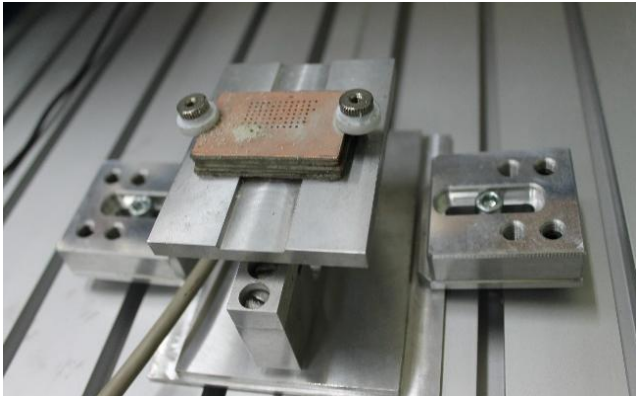
Fig. 3. Instrument for measuring axial efforts
