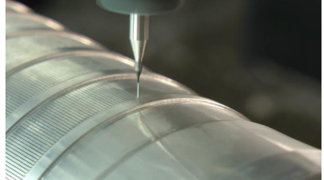
Fig. 1. Micro-drilling with micro-drills on the CNC machine of the firm DATRON
