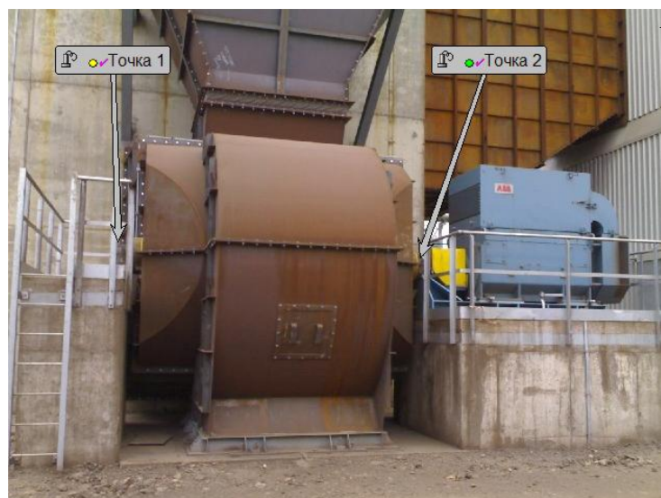
Fig.1. The impeller of the main exhaust fan mounted in the bearing housings with control points of vibration.
